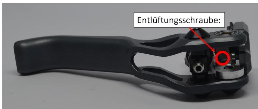
Possibly, so far reduced lever length of the lever that the nipple can be turned in completely and does not conflict be hexagonal with the lever. Repeatedly press the brake lever slightly. In the brake lever reach possibly the master piston adherent air bubbles in the reservoir. From then do not press the brake lever!
