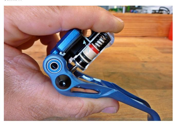
In the following step, the bleeding of the secondary chamber of the brake pump will be described. Since there was no need for an additional hole between secondary chamber and expansion tank for reasons of space, this is a major step.
