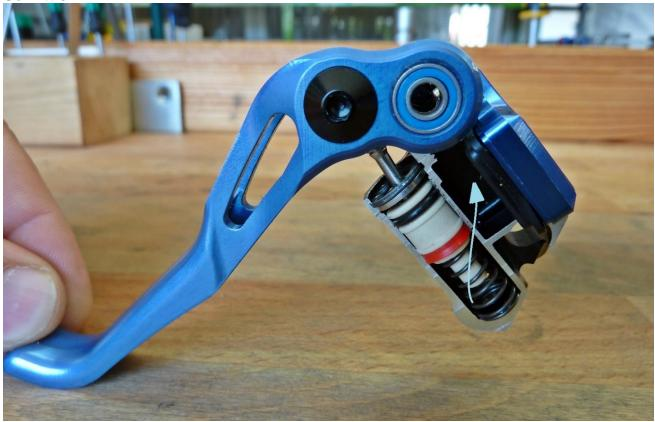
Hold the master cylinder in the position shown and push / pull the syringe a few times. The sniffer holes form the highest point oft he high pressure chamber – any air in the high pressure chamber migrates into the expansion tank and thus into the syringe.
