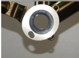
2) Plug the eccentric bearings cap without clamping bolt unit onto the steel caps. Mount the greased clamping bolt. Fix the clamping bolt with the M4 screw slightly.
