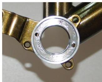
1) Screw the steel bottom bracket caps firmly into the frame by using the special EX-Tool. Make sure the tool fits firmly to the ground of the cap. Torque: 40 Nm.
