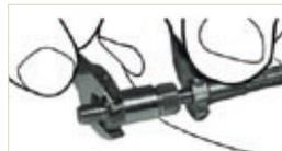
3. Fit the other end of the assembly, and attach to the lever. Thread the M6 adapter into the caliper and then tighten the M8 swivel male into this.
