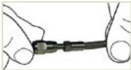
3. Push the threaded spigot of the fitting into the hose, ensuring that it pushes into the centre bore. Turn the hose clockwise to engage the thread by hand until the face of the collar reaches the shoulder of the fitting.
