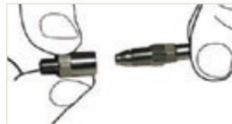
1. Take the M6 adapter (left) and thread the M8 male into it, tighten with spanners. (For M8 swivel fitting direct to calipers or master cylinders refer to General Fitting Tips below)
