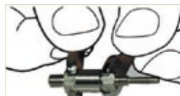
2. Using an 8mm spanner on the collar, tighten both pieces complete onto the hose as described in (fig. 5).
