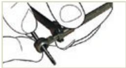
5. For banjo fittings, use an 8mm spanner on the collar and insert a screwdriver or bar through the banjo head, tightening the fitting in a clockwise direction to engage the second locking thread until the face of the collar reaches approximately 1.5mm from the shoulder of the fitting **-DO NOT OVER TORQUE-**
