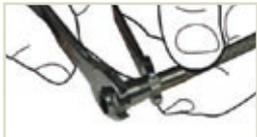
4. With an 8mm spanner on the collar, tighten the fitting in a clockwise direction to engage the second locking thread until the face of the collar reaches 1.5mm from the shoulder of the fitting. **NB. Do not fully tighten the fitting to meet the shoulder as this can lead to over-tightening**
