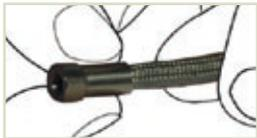
2. Gently push the collar onto the hose, feeding the steel braid into it by rotating the collar as you push it on.
