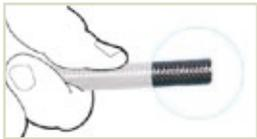
1. Cut hose to suit your system, using sharp cable cutters or a small hacksaw with sharp blade.
