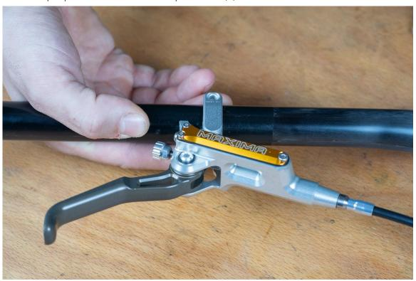
3. Apply a small drop of medium strength thread locker (e.g. Loctite 243) to the short clamp screw (9). Tighten the screw with 1-2 turns so that the clamp does not fall apart. Proper tightening takes place later.
