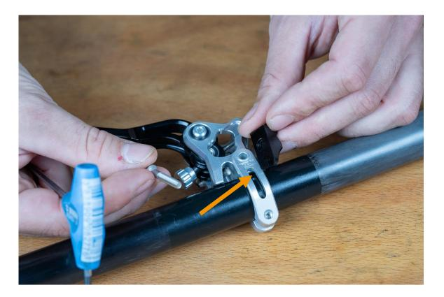
5. Insert the M5x8, Torx25 bolt <u>with washer</u> (3a) into the Shimano I-Spev EV compatible shift lever (4). <u>Note:</u> It is important to use the washer (3a), otherwise the interface will not work properly!
