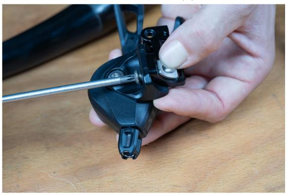
5. Apply a small drop of medium-strength thread locker (e.g. Loctite 243) to the end of the long clamp screw (10) and insert it into the interface (1). Fasten the interface (1) with the long clamp screw (10) on the bottom side of the clamp, the tightening will take place later. Pay particular attention that the orange marked connector of the interface adapter sits correctly in the intended notch of the CNC clamp.
