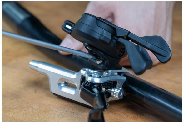
7. Align the pump on the handlebar as required. Then tighten the <u>upper</u> clamp screw (9) with a maximum torque of 1.5Nm.
