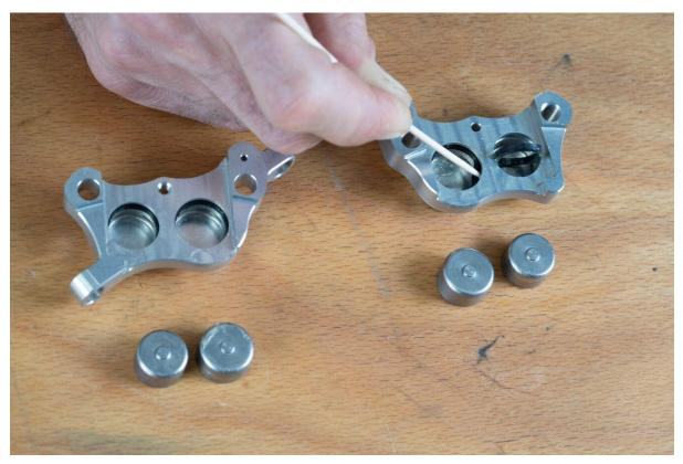
7. Clean the caliper halves with warm water and a liberal amount of washing-up liquid. Works best in combination with a soft brush and a lot of clean water for rinsing afterwards. Before assembly, make sure everything is properly dried and no water residue remains. You can dry the caliper halves with compressed air or by putting them on a household radiator for some time.
